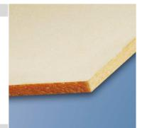
AIREX<sup>®</sup> C71 is a closed cell, cross-linked polymer foam especially formulated to maintain its stability also at higher processing or service temperatures.
